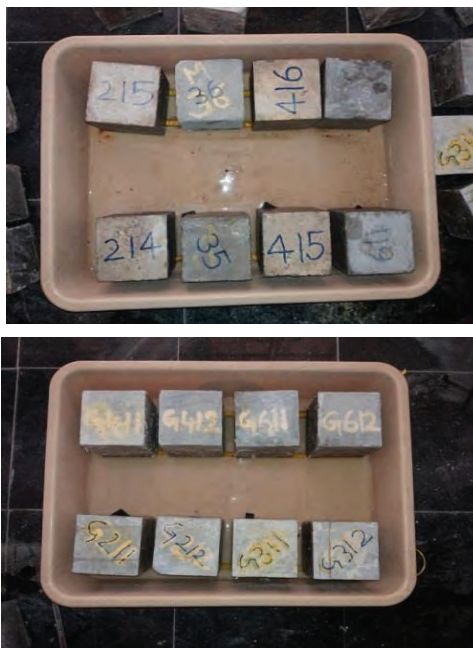
Figure 8. Testing of SCCP and GFRSCC Specimens for Sorptivity
