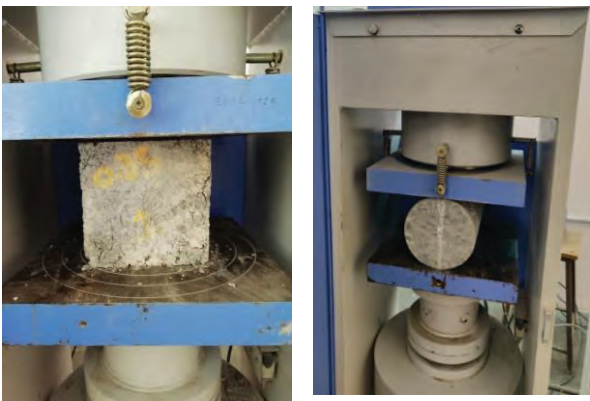
Figure 7. Compressive strength test and Split tensile test of LECAC50 cube and cylindrical specimen respectively with Automatic compression testing machine of 2000kN capacity
