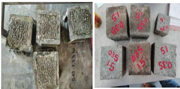
Figure 3. Casting of cube specimens
