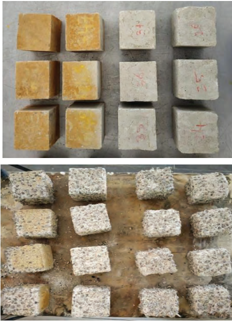
Figure 7. After Immersion of Specimens in Acids and Sulphate
