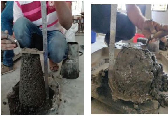
Figure 6. Workability test of LECAC50 using Slump cone test
