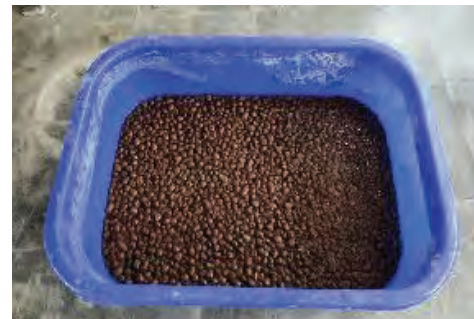
Figure 5. LECA Water absorption test
